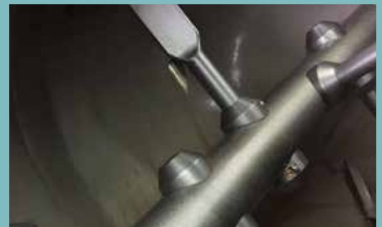
View of the Conch after 15 minutes of intensive cleaning in circulation. Fat 5 - 8% of the net volume of the Conch.
